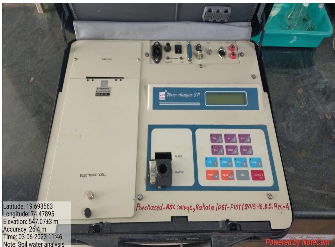
Photo: Soil Water Analysis Kit System in the Chemistry Department.
